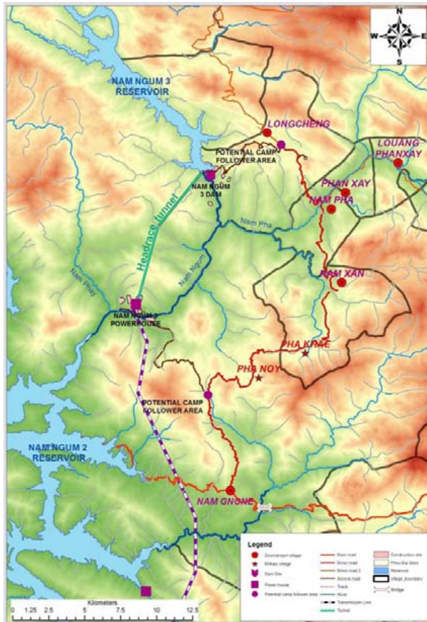
Figure 1: NN3 Dam Site and Access Road.
